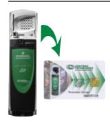
Drive automatically writes to the SMART(41(1)) when a parameter save is performed
