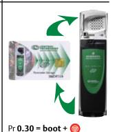
Drive boots from the SMART(4.1(1)) on power up and automtically writes to the SMART(4.1(1)) when a parameter save is
