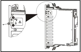
1. Internal EMC filter. Remove the bottom screw as shown.
