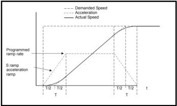
Since the ramp rate is defined in s/100 Hz or s/1000 rpm and the S ramp parameter is defined in  $s^2/100$  Hz or  $s^2/1000$  rpm, the time T for the 'curved' part of the S can be determined from:
