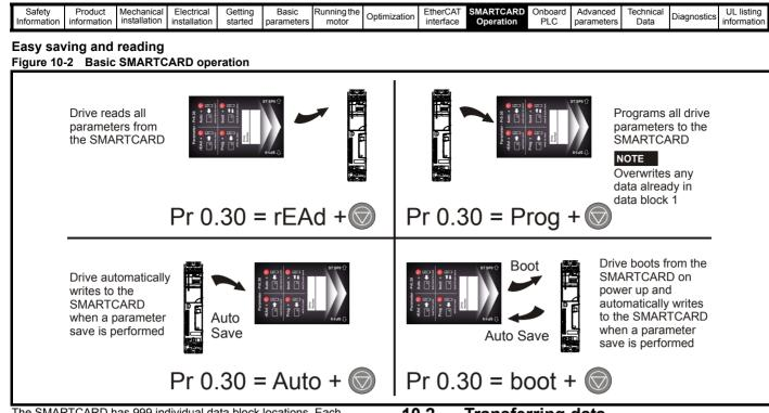
The SMARTCARD has 999 individual data block locations. Each individual location from 1 to 499 can be used to store data until the capacity of the SMARTCARD is used. The drive can support SMARTCARDs with a capacity of between 4kB and 512kB.
