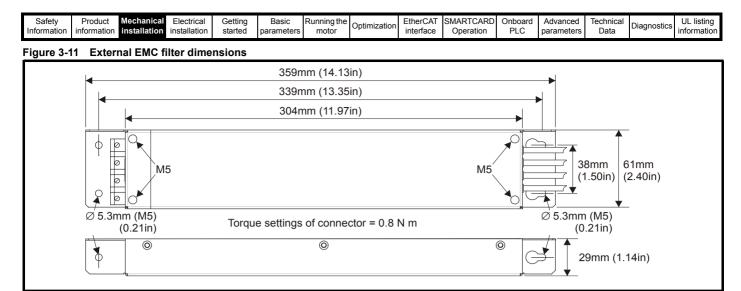
Figure 3-11 shows a 3 phase filter. For a single phase filter, there are only 3 input terminals (L1, N, ground) and 3 output cables (L1, N, ground).
