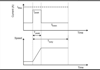
This is a profile with acceleration/deceleration periods where the peak output current from the drive ( $I_{peak}$ ) is given as a proportion of the base current ( $I_{base}$ ) for a defined period of time. ( $T_{peak}$ ).
