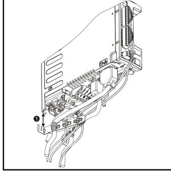
Grounding bracket and drive to be directly connected to a grounded backplate.
