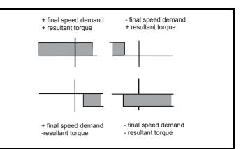
This mode of operation can be used where torque control is required, but the maximum speed must be limited by the drive.
