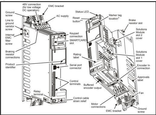
\* The Marker Tag (as shown in Figure 2-3 above), is where markers can be placed to identify a particular drive which can prove beneficial where several Digitax ST drives are located in the same panel.
