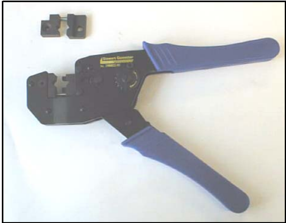
Figure 1-2 Stewart Ferrule Crimp Hand tool and 5.2mm Cable Crimp
