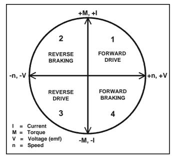
Figure 3-4 The four quadrants of the DC motor torque-speed diagram
