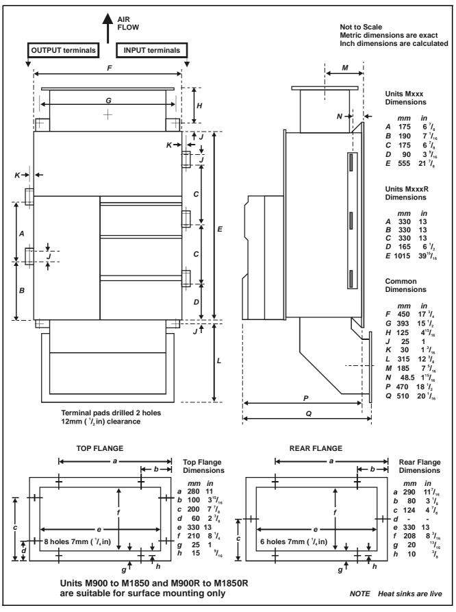
Figure 5-5 M900(R) to 1850(R) Drive Dimensions
