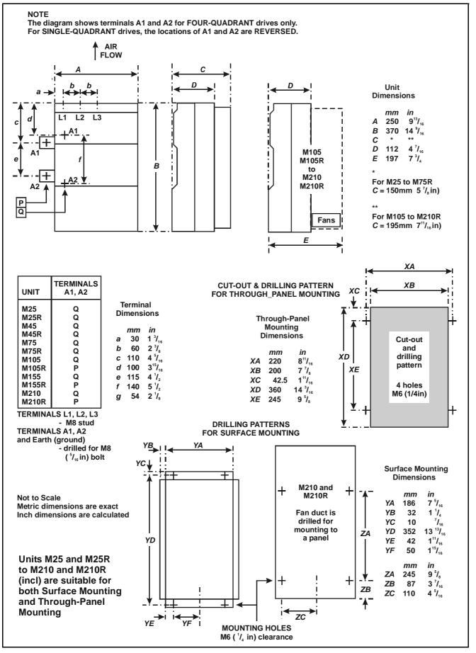
Figure 5-3 M25(R) to M210(R) Drive dimensions
