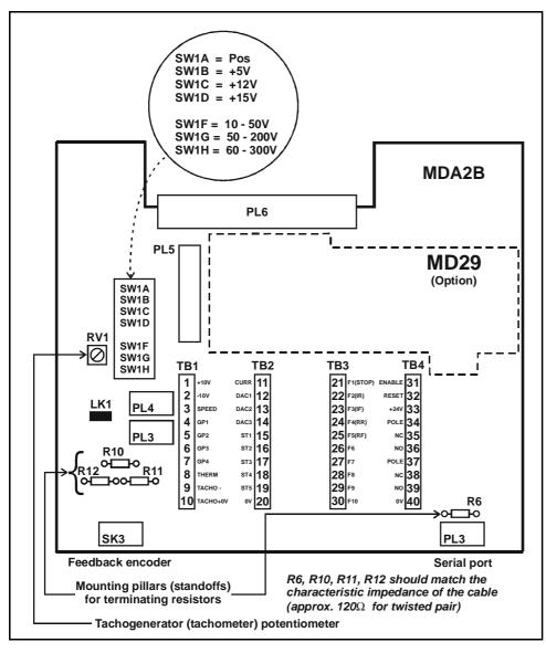
Figure 6-4 Location of principal components on PCB MDA2B issue (revision) 2
