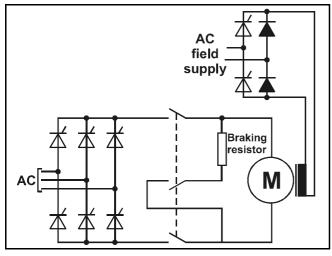
Figure 3-5 Typical arrangement for dynamic (resistive) braking of a "single-ended" DC drive
