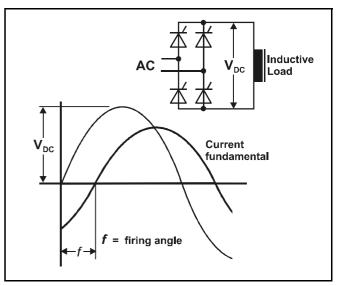
Figure 3-1 Behavior of a single-phase fully-controlled thyristor rectifier (SCR) supplying a highly-inductive load
