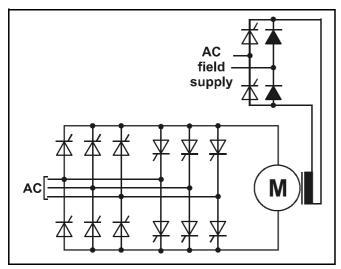
Figure 3-3 Dual bridge or parallel-pair 3-phase thyristor (SCR) arrangement for a 4-quadrant DC motor drive
