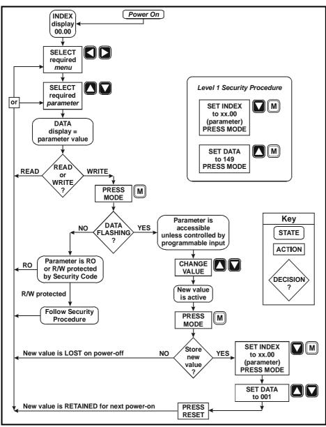
Figure 8-1 Adjustment of parameters and level 1 security
