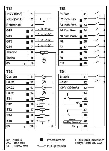
Figure 6-5 Control connections
