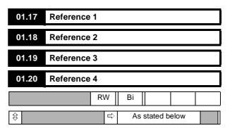
Reference 1, parameter **01.17** is the default destination of the external speed reference (terminal TB1-3) through the programmable input **07.15**.
