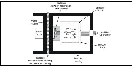
An example of this is the Unimotor, where isolation from the motor is achieved by inserting a plastic mounting plate between the motor housing and encoder housing and a plastic insert fitted in the motor shaft for encoder mounting to the motor shaft. With this preferred method of mounting, noise currents are prevented from passing from the motor housing into the encoder housing, and hence into the encoder cable.
