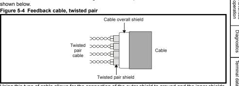
Using this type of cable allows for the connection of the outer shield to ground and the inner shields to 0V at both the drive and encoder.
