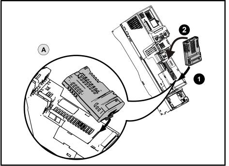
Option module slots must be used in the following order: (Slot 3), (Slot 2) then (Slot 1).
